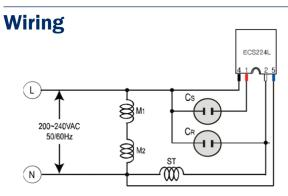
Cs: Start capacitor, Cr: Run capacitor, M1/M2: Main coil, ST: Auxiliary coil
