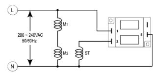
M1/M2: Main coil, ST: Auxiliary coil
